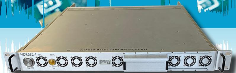
An internal ARM A8 microprocessor running embedded LINUX is used for command/control of the unit via an Ethernet interface and power is derived from a 115 VAC external power supply input (power consumption is 100 Watts). The unit is housed in a 1U, 19 inch equipment frame with 19"x18"x1.75" overall dimensions that provides RF shielding, thermal management, and protection suitable for harsh environments.
